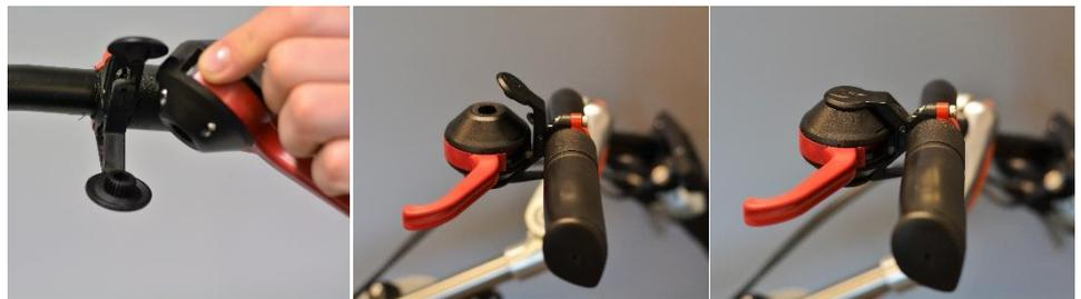
Place the control in the bracket in the desired position. To remove the lever when charging, reverse the process
