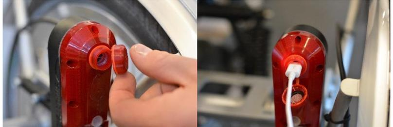
Turn counterclockwise to open the charging cover. Use the USB charger incl. in the kit
